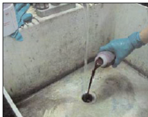
Figure 63: Dye Testing Plumbing (NIWPC, 2003)
