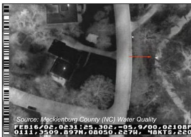
Figure 74: Aerial Thermography Showing Sewage Leak
