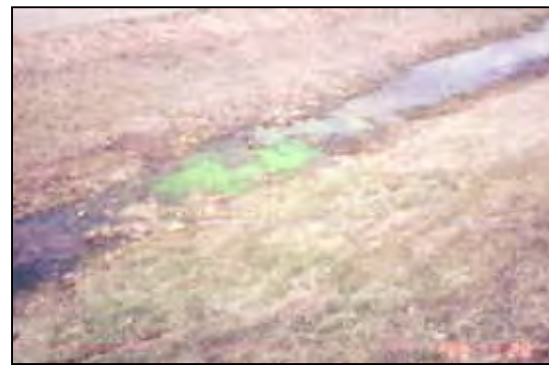
Figure 73: Dye surfacing in a septic field
